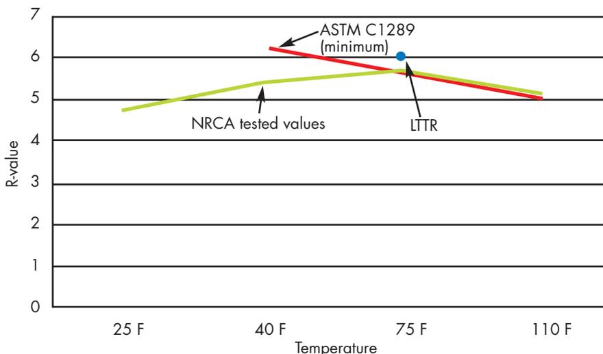
NRCA's tested data, LTTR and ASTM C1289's minimum required R-values
